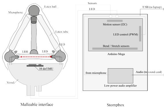
**Figure 3:** An outline of the system. On the left, a section of the malleable controller; on the right a schematization of the stompbox.
